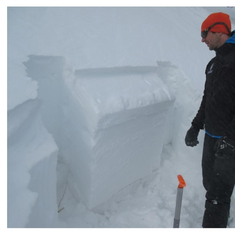
In this pit we had multiple layers propagate in our stability tests. Two wind slabs near the surface, and a thin layer of facets above the hard crust on the ground. ESE aspect at 9,000' near Fairy Lake. Photo: GNFAC
