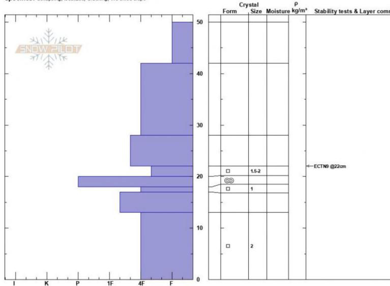
Where the collapsing was happening, the slab over the weak layer was thicker and about 4F hardness. HS approx. 75cms.
