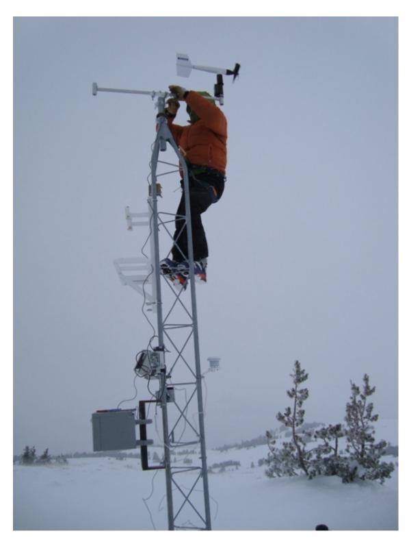
With numb fingers, Mark Staples puts up the weather station at LuLu Pass outside Cooke City. It was a frigid 2F with a 20 mph wind. It measures wind speed, direction, temperature and relative humidity. This new station was recently purchased by the **Friends of the Avalanche Center**. It sends data hourly to a web page: <a href="http://bit.ly/5yXgti">http://bit.ly/5yXgti</a>
