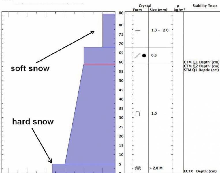
This snowpit was recorded in the northern Gallatin Range just east of Hyalite Canyon. Notice the strong, hard snow near the ground and soft, low density snow near the surface. Stability tests show fractures about 10 inches down. While not a problem in this snowpit, they would be a concern if a denser wind slab were deposited on top of this snowpit. Image: A. Marienthal
