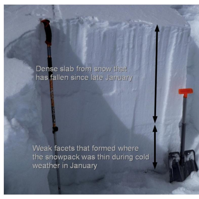
There are two basic snow structures in the Bridger Range. One is a deeper snowpack that has a several thin layers of facets in the middle of the snowpack but these are not much of a concern. The other basic structure is shown in the photo. While these areas have adjusted to the weight of new snow, making avalanches less likely, this is a poor structure which keeps avalanches possible. Photo: GNFAC
