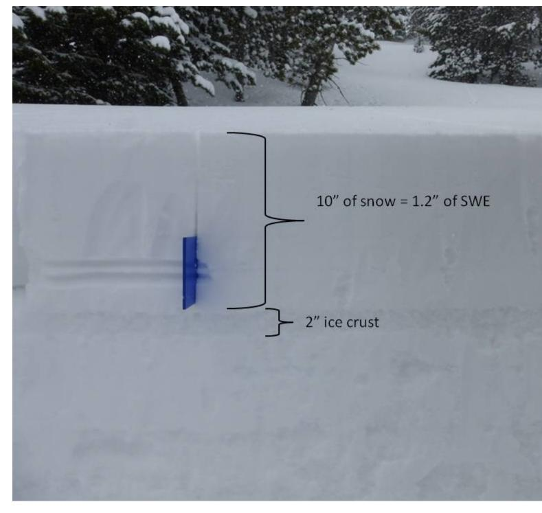
Two separate storms over the past five days have deposited up to 10" of snow around the Big Sky area. These two storms combined to equal 1.2" of SWE. Although the new snow is well bonded to the hard underlying ice crust, wind slabs remain a concern. Loose, wet avalanches will also be a concern when the sun comes out. Photo GNFAC
